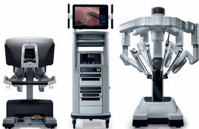
Full robotic set up including console, screen and robotic arms
